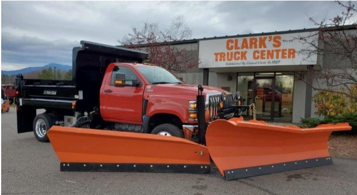
International CV515 with front plow & wing plow
