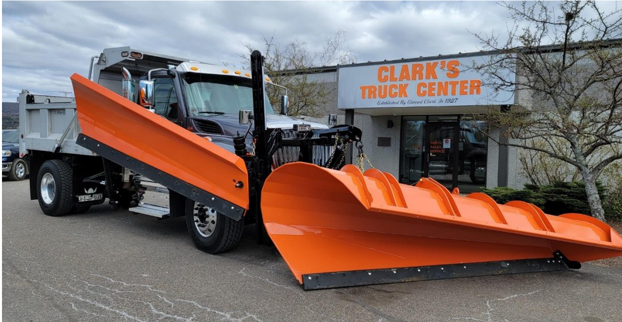
2022 International HV507SFA Truck with front plow & wing plow (ordered in July 2021, delivery expected in 8 weeks, ours will be red)
